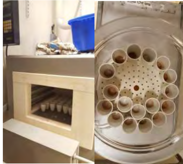
Furnace for soil organic matter
