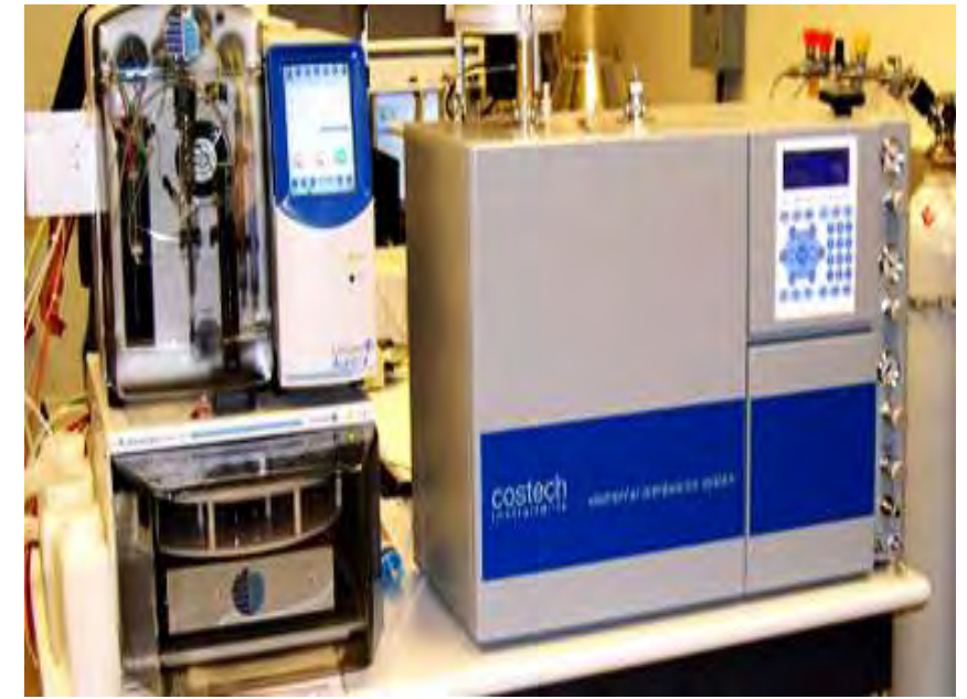
Elemental Analyzer - Isotope Ratio Mass Spectrometer (EA-IRMS) for soil C, N and C/N
