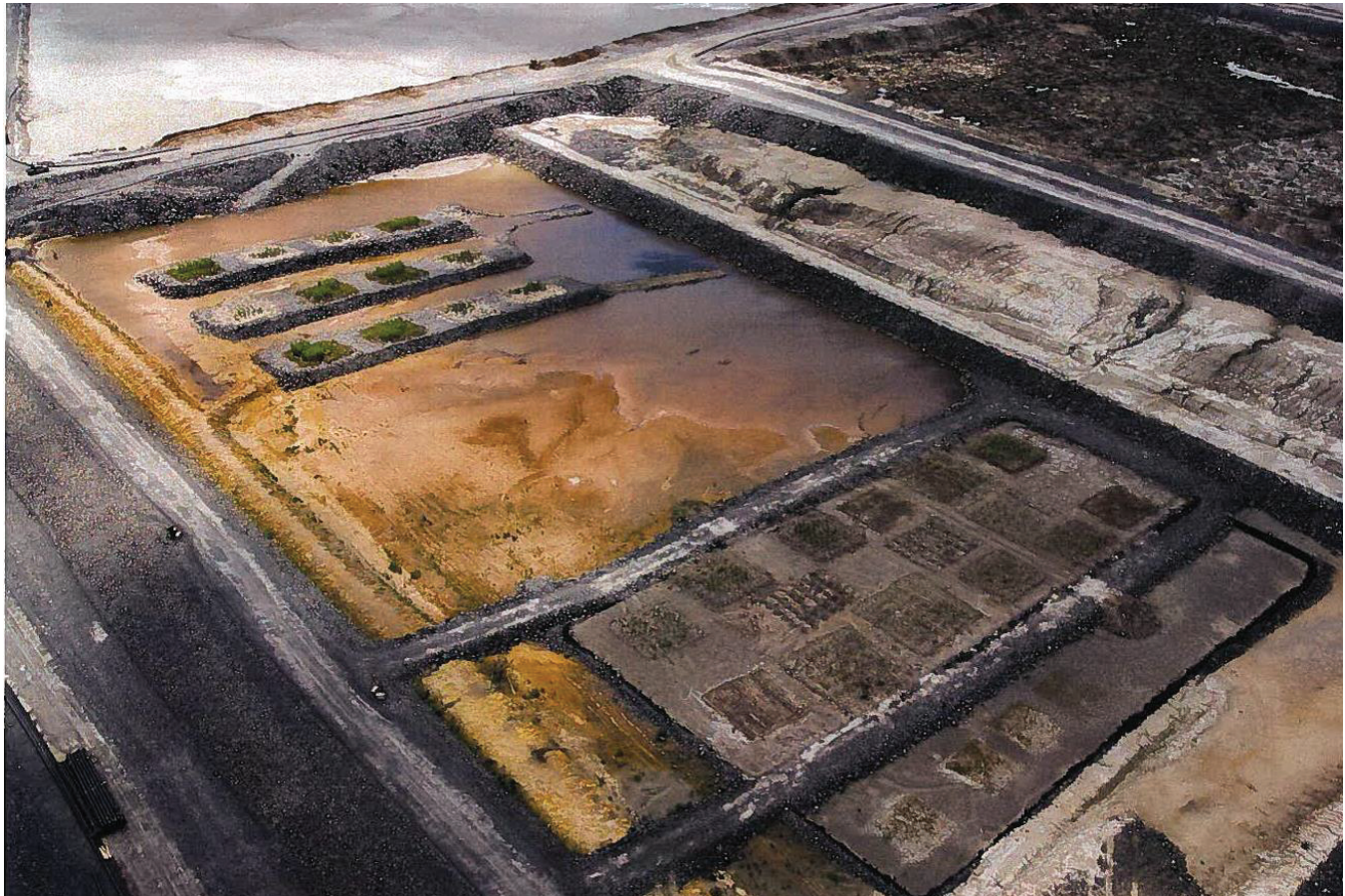
FIGURE 1. Experimental zone in the tailings facility of the Canadian Malartic mine (property of Canadian Malartic Partnership): experiment 1 on waste rock at the upper side, and experiment 2 on thickened tailings at the lower side.
