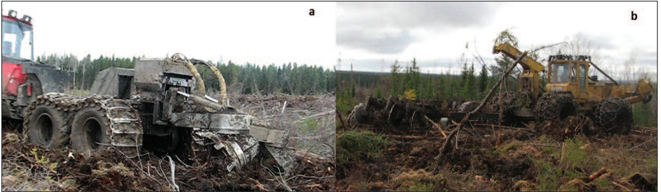
**Fig. 1. (a)** T26 Scarifier, a machine with two large, robust toothed discs. It is the most used site preparation machine in the boreal forest. **(b)** Forest harrow, multi-disc toothed machine, aligned in two rows. In Abitibi, it is used to prepare the clay soil forest sites and waste lands.
