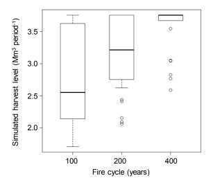
**Figure 2.** Box and whiskers plots representing the probability distributions of the simulated implementation of the optimal solution (3.8 Mm<sup>3</sup> period<sup>-1</sup>) provided by the timber supply model (Equations (1)–(6)) under current (400 years) and probable interval for future fire regimes (100 and 200 years).
