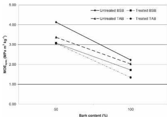
FIGURE 2. Effect of hot-water treatment of black spruce (BSB) and trembling aspen (TAB) bark on the specific modulus of elasticity (MOE<sub>spec</sub>) of particleboard made from black spruce and trembling aspen bark.
