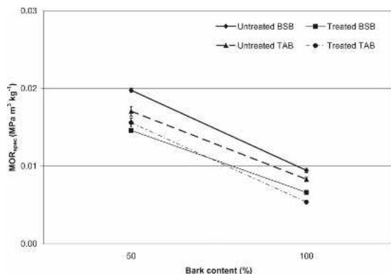
FIGURE 3. Effect of hot-water treatment of black spruce (BSB) and trembling aspen (TAB) bark on the specific modulus of rupture (MOR<sub>spec</sub>) of particleboard made from black spruce and trembling aspen bark.
